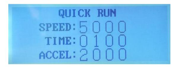
Press button to choose and set SPEED, TIME, ACCEL, Press to modify the corresponding data, finish setting, long press "set" button back to the main interface
