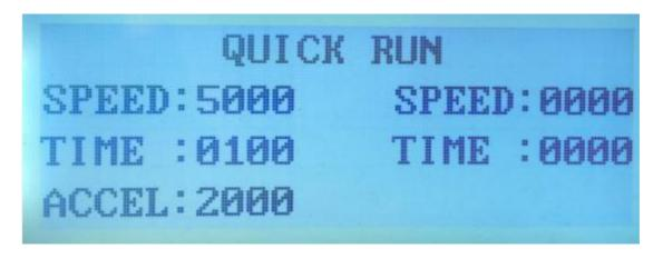
Long press "set" button to enter parameter setting interface as below:
